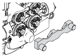
3. Rotate all of the triangular rings to the unlocked position.
